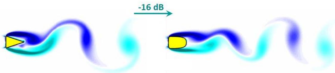
**Figure 1: optimal shapes for aeroacoustics: Vorticity field in the laminar flow over 2D bodies. The left geometry radiates 45 times more acoustic power<sup>2</sup>.**
