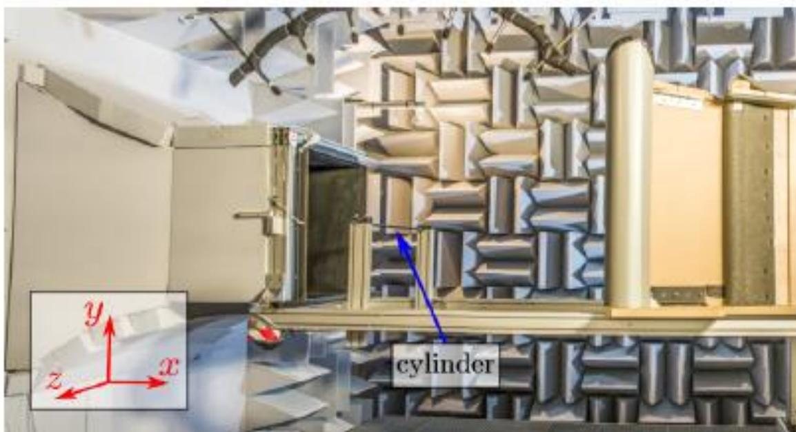
Figure 2: Anechoic wind tunnel facility BETI at Institut PPRIME. Acoustic antenna at the top.
